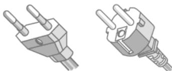
In Indonesia the power plugs and sockets are of type C and F. The standard voltage is 230 V and the standard frequency is 50 Hz. The Type C is also known as the standard "Euro" plug while Type F is also known as "Schuko".
