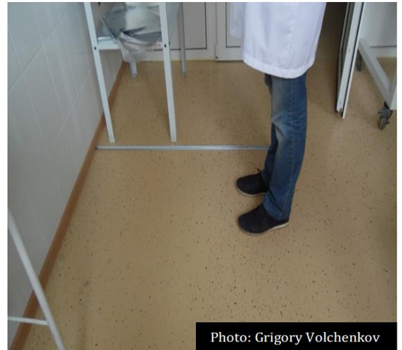
Figure 5 (above) Illustrates use of measurement tape to indicate 1 m distance from the back of the GUV fixture to the sensor. Detector (left) is raised and lowered to find maximum output (irradiance) of the UV beam for recording output. If allowed, permanent marker on the floor would facilitate repeat measurement. Or use as a yard/meter stick between the face of the fixture and the GUV radiometer's detector.
