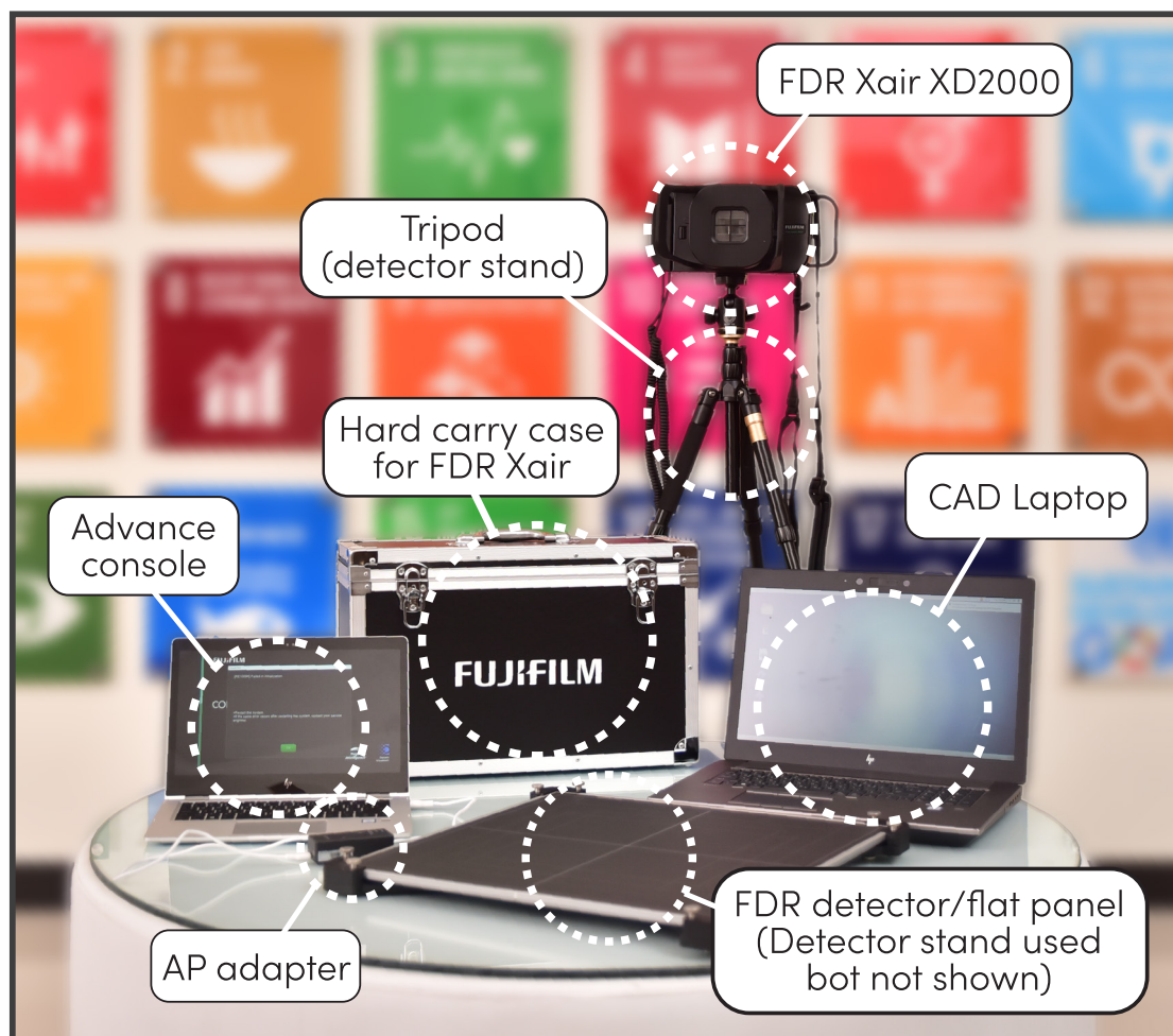
Figure 12 Labelled Fujifilm FDR Xair core system. Image courtesy of DOPASI.
