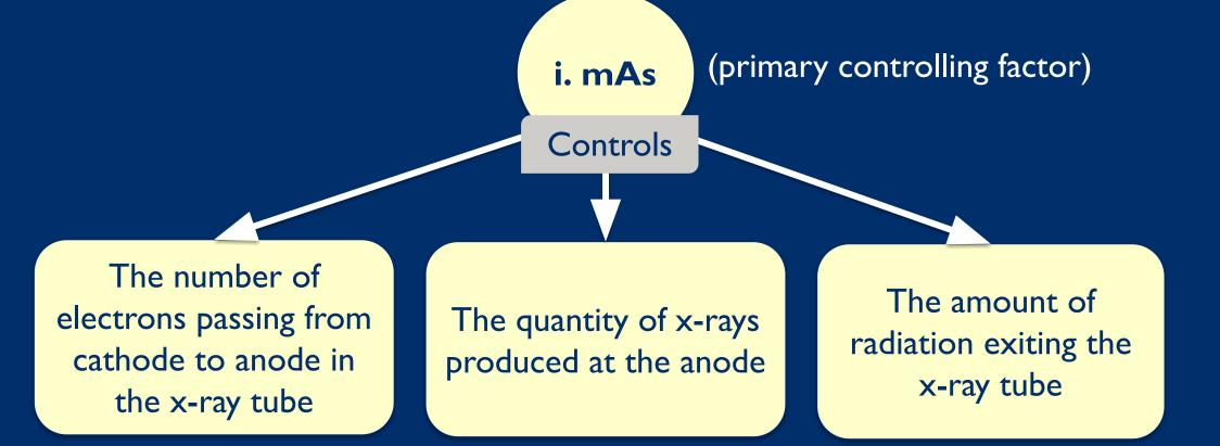
\* mAs controls density by controlling the quantity of x-rays emitted from the x-ray tube and the duration of the exposure. \*\* Doubling the mAs doubles the quantity or duration of x-rays emitted, thus doubling the density on the film.
