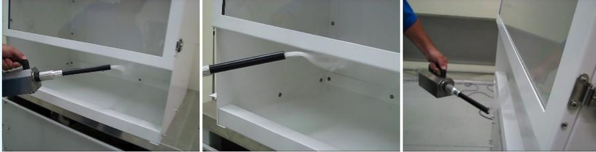
Smoke inflow test
