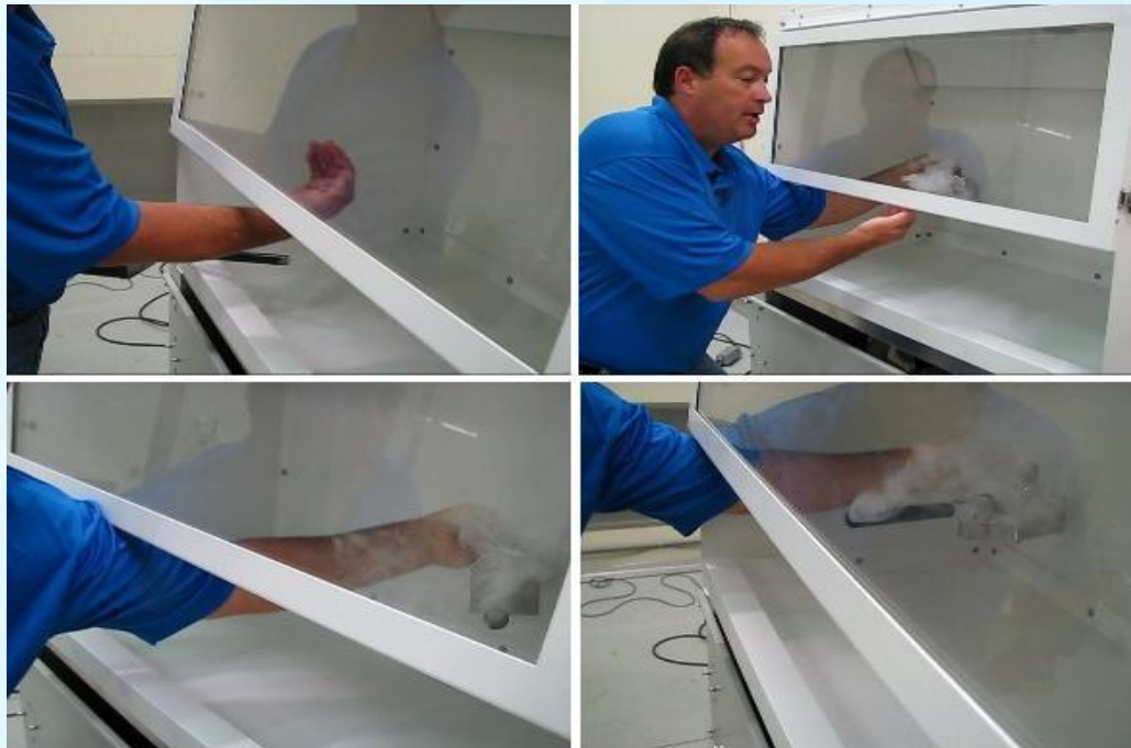
Smoke outflow test
